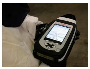
*Thermo Scientific's microPHAZIR AS can provide ACM identification in seconds*
