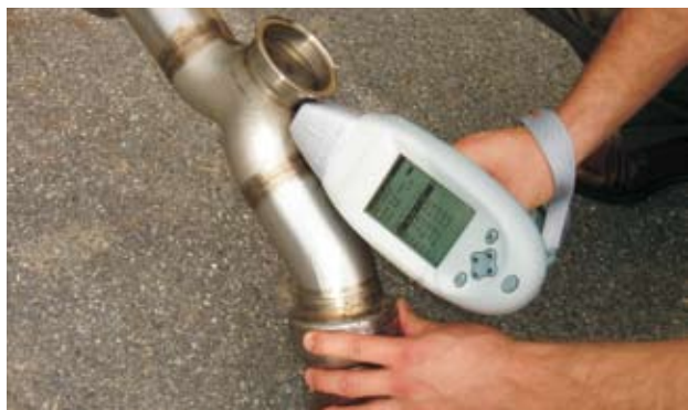
Thermo Scientific NITON Analyzers can be used to analyze all components in the system, even to verify the dilution ratio of finished welds.
