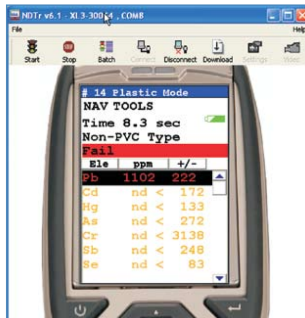
Figure 2. Example of “Fail” for lead in Plastic Mode, Non-PVC Type sample, though inconclusive for six other displayed elements of interest, tested at 8 seconds
