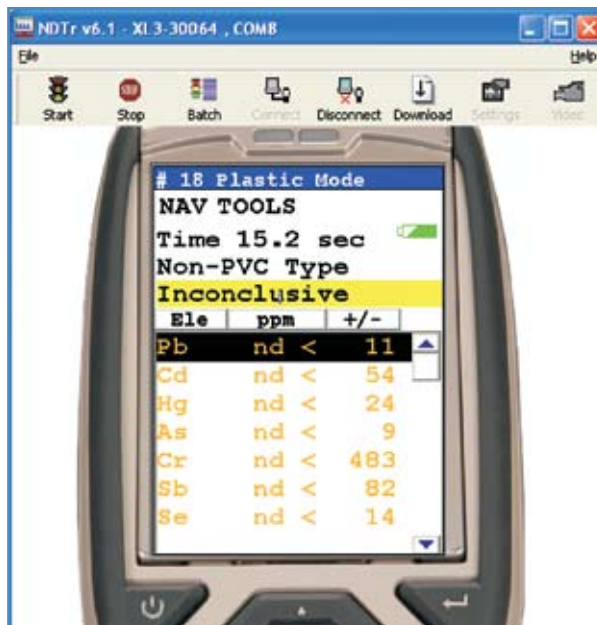
Figure 4. Example of "Inconclusive" for all elements of interest in Plastic Mode, Non-PVC Type sample, tested at 15 seconds
