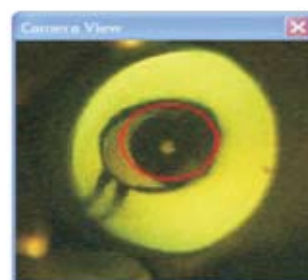
Figure 1: Eye feature on a painted object through the lens of the NITON analyzer CCD camera.
